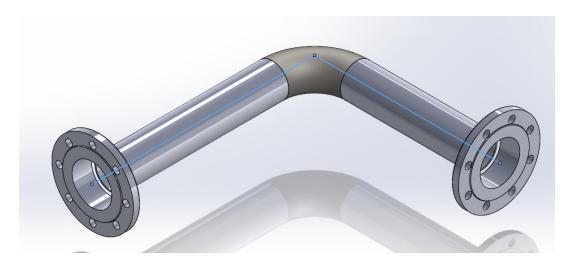
If end components are also defined in the same pipe specification, these are not used when generating the pipeline, since the QuickPlace method Spool Flange now has the <a href="https://example.com/higher-priority">higher priority</a> by default.
