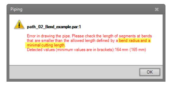
A **180° bend** requires a minimal **technical tolerance of exactly 0.01 mm.**Therefore, the length of the line segment must be **2x bend radius + 0.01 mm**.
