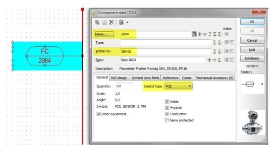
This new symbol type was introduced to give users the option of differentiating symbols for process control technology (PLT, for sensors and process control functions) from regular P&ID symbols.
