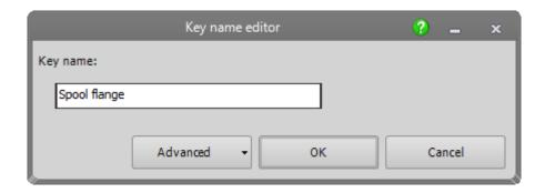
When generating a pipeline with Smap3D Piping, 3D components defined in a pipe specification with the key name **Spool Flange** are always placed on a free (unconnected) pipeline end in order to automatically create <u>Spool pipelines</u>.
