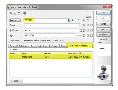
Mechanical accessories can be added to a component in different ways in P&ID:
